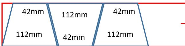
Insulation cut pattern for 90° bend
