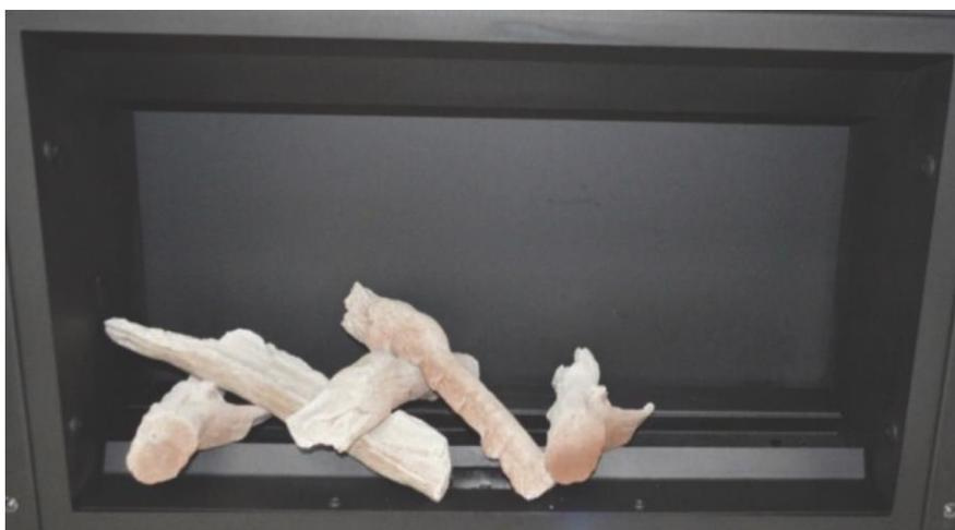
f) Place 2nd log No. 2 log onto branch log, use location grooves to locate.
